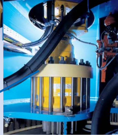
Modular designed slewing gear drive unit
