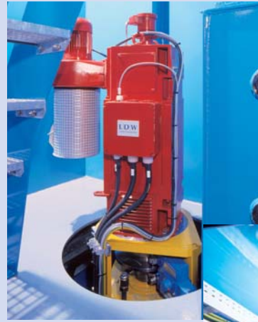
Modular designed slewing gear drive unit
