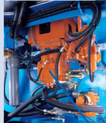
Hydraulic unit driven by an AC motor
