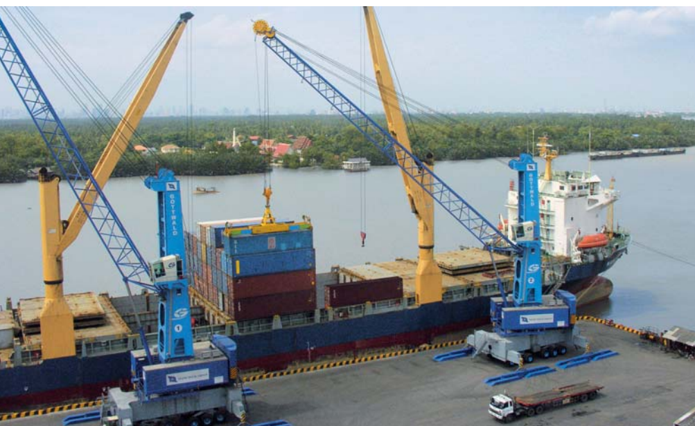
HMK 260 E cranes at Thai Property Terminal, Bangkok, Thailand: crane stabilisers are adapted to quay specifications
