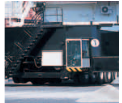
Additional cab on the chassis
