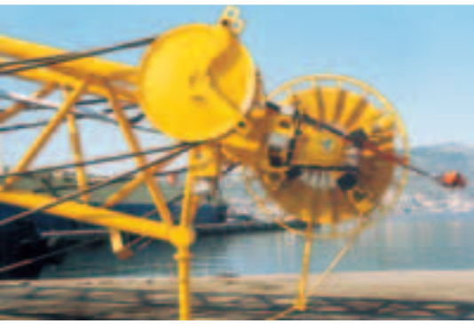
Cable reel on the boom head
