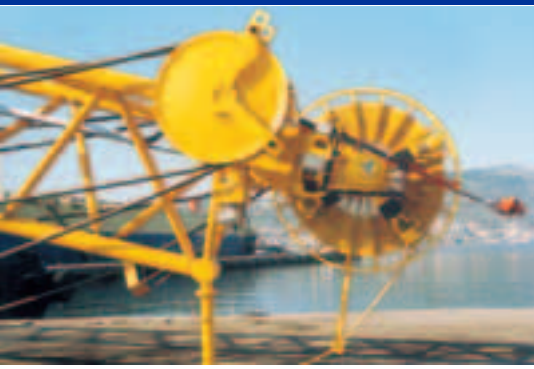
Cable reel on the boom head
