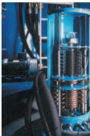
Slip ring assembly for external power supply
