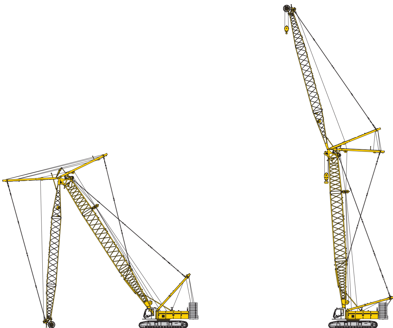
Erecting of main boom and luffing jib
